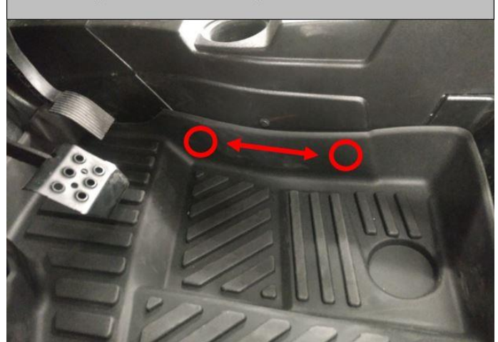
Rivet placement into side portion of the floor mat.
