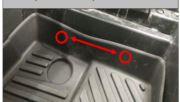
Rivet placement into rear portion of the floor mat.
